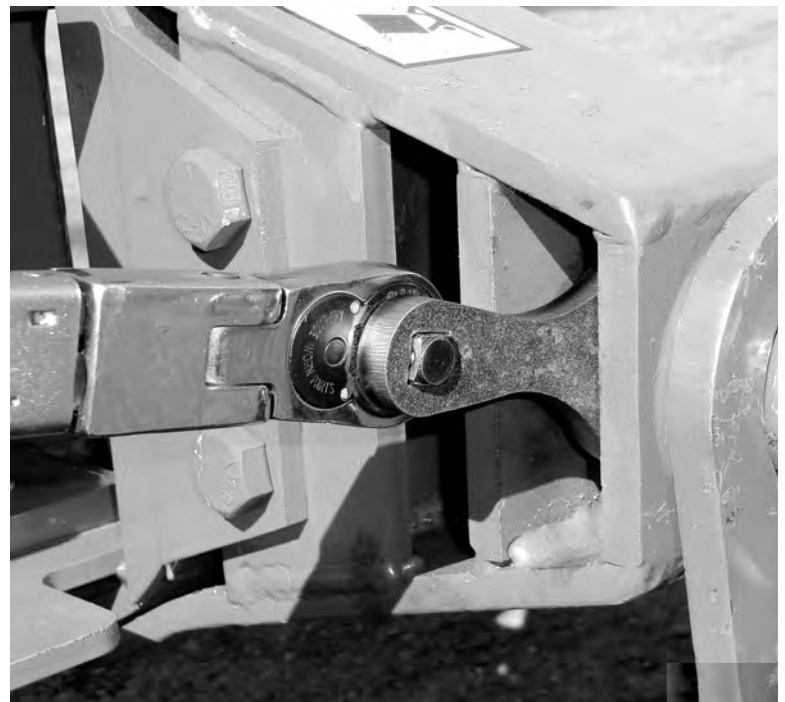
Pin wrench is installed on the torque wrench in-line
