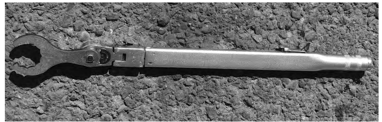
Pin wrench is installed on the torque wrench in-line
